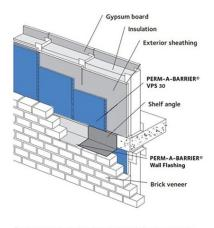
Typical vapor permeable air barrier application drawings are for illustration purposes only Please refer to gcpat.com/construction for specific application details.
