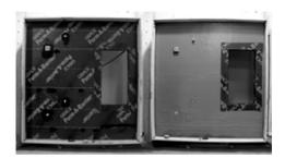
The mock-up is exposed to positive and negative sustained wind loading of 12.5 psf (600 Pa) for a one-hour duration in each direction. The wind gust loading reaches 25 psf (1200 Pa), which is equivalent to wind gusts of 99 mph, again in both the positive and negative direction. After all of the wind loading is completed the air barrier assembly is measured for air leakage in both the positive and negative direction.
